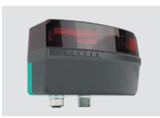
The R2300 offers four scanning layers in only one LiDAR sensor and therefore highly accurate 3-D measurement. The integrated red pilot laser can be switched on and adjusted to the scan planes of the infrared measurement laser, enabling direct alignment of the sensor. The R2300 has no moving parts, which makes it especially durable in harsh environments. The sensor's compact housing even makes installation in tight spaces possible.
