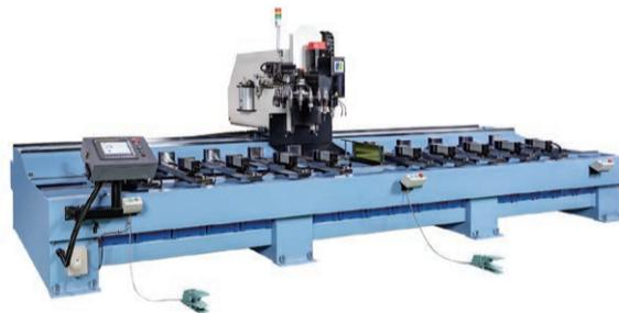
The 'FB-5000-20ATC-S' is a high-torque steel processing machine with enhanced rigidity, ideal for cutting square pipes and H-beams. At JIMTOF 2024, we'll demonstrate its high-speed capabilities in partnership with Nachi-Fujikoshi.
