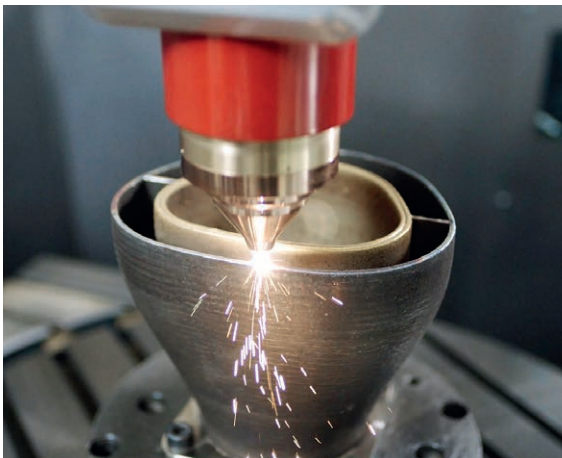
There has been progress in the combining of machine tools, such as a tool for laminating shapes with a cutting tool (provided by DMG MORI CO., LTD.)
