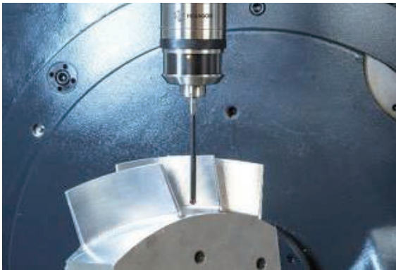
On-machine measurements of objects being machined enables the consolidation of processes and enhances precision (provided by Captain Industries, Inc.)
